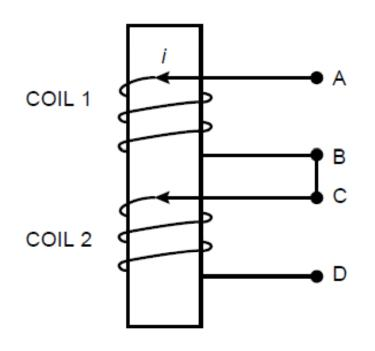
If the winding between terminals A and D are considered as a single circuit having a self inductance  $L_A$  henrys then if the same increase in dt seconds is di amperes then the e.m.f. induced in the complete circuit is
